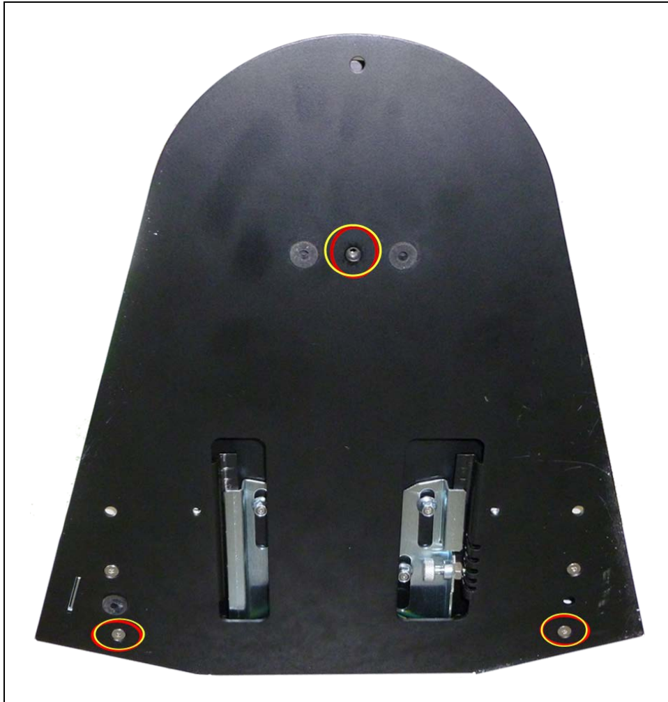
Figure 3-22. Underside of Docking Station Foot, Showing Screw Locations
