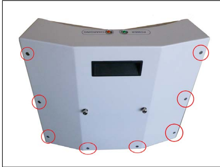
Figure 8-9. Docking Station Rear Cover Screws (8 of 10)
