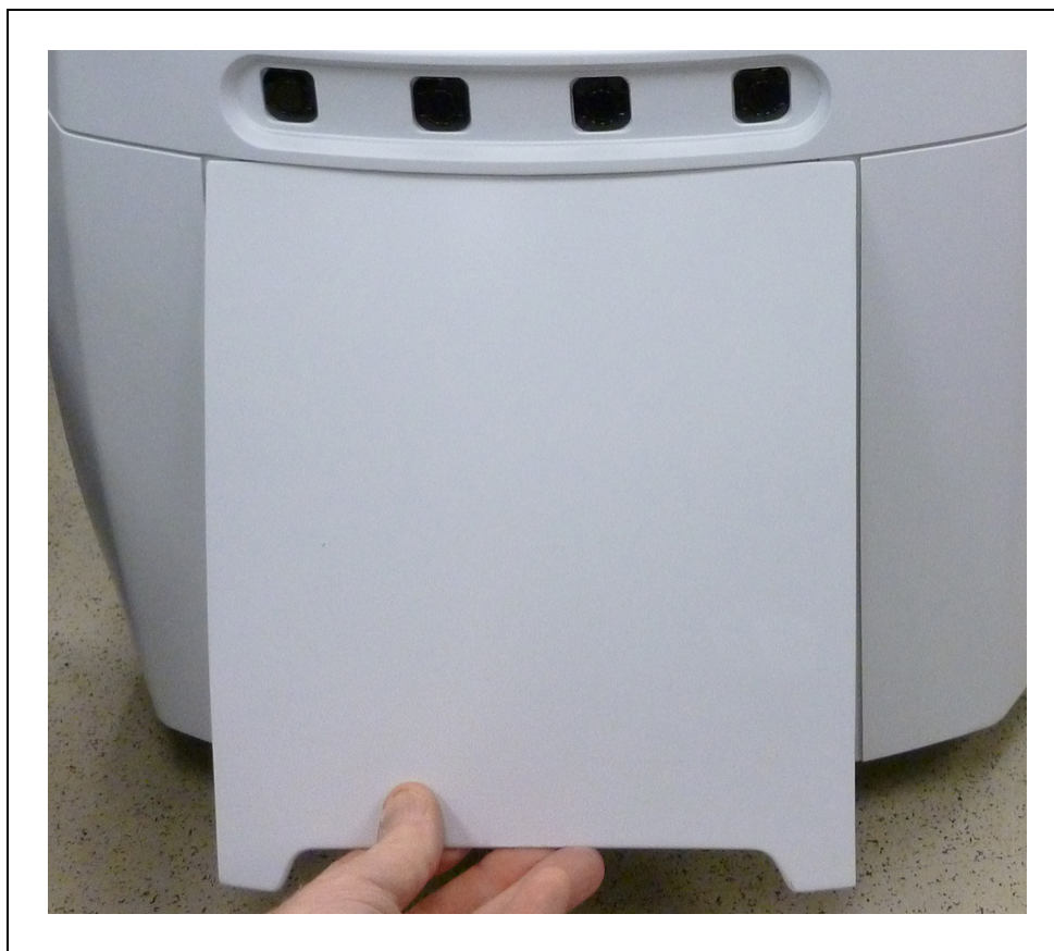
Figure 3-14. Pulling the Bottom of the Rear Platform Cover Out
