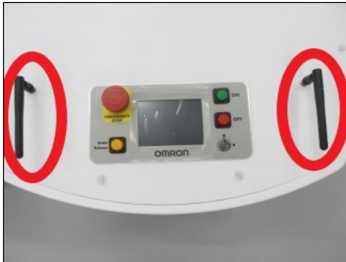
Figure 3-11. Robot Antennas Circled in Red
