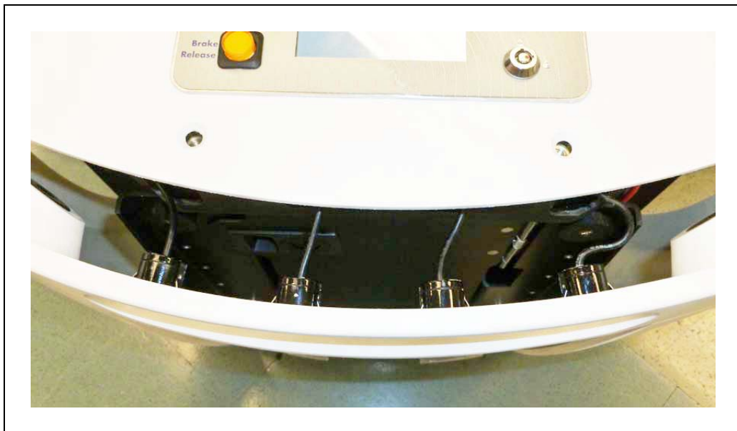
Figure 8-20. Sonar Leads, with Connectors Still in Chassis
