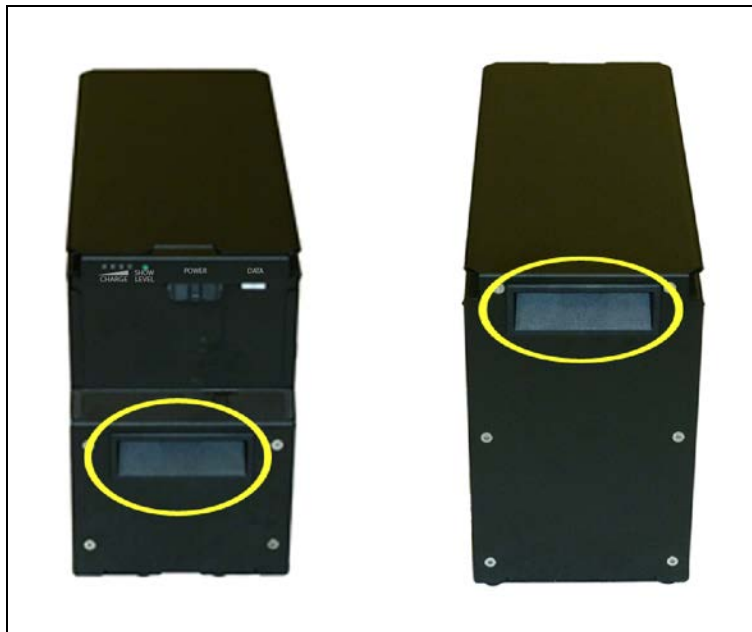
Figure 3-16. Battery Recesses, for Gripping
