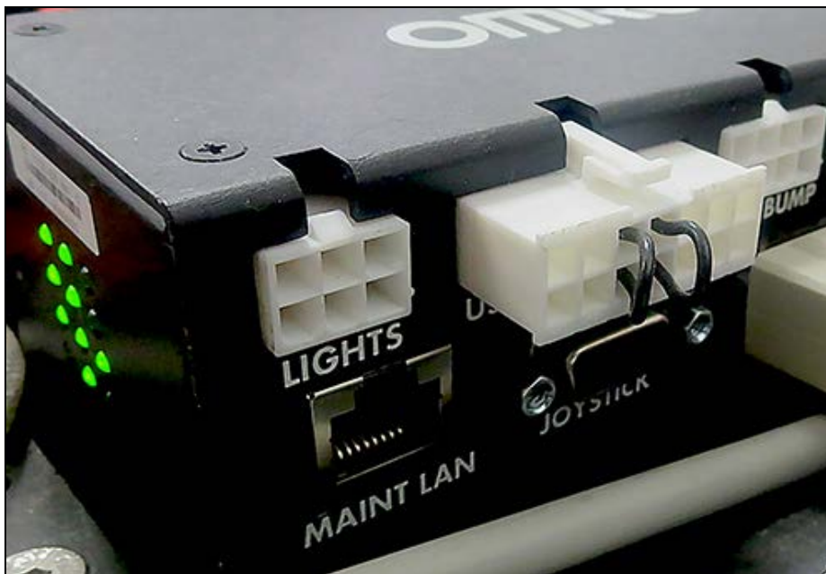
Figure 3-19. E-Stop Jumper on LD Platform Core
