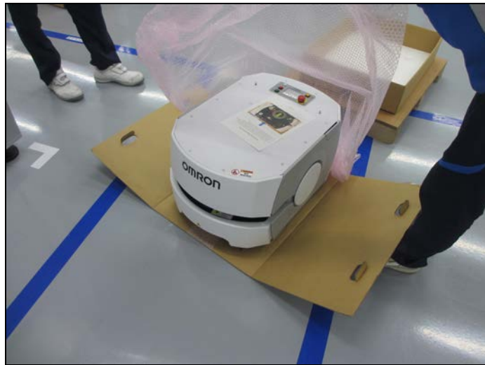
Figure 3-9. Protective Plastic Sheet Being Removed
