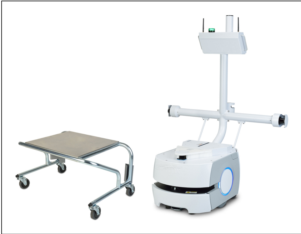
Figure 1-1. Cart and LD Platform Cart Transporter, Separate
