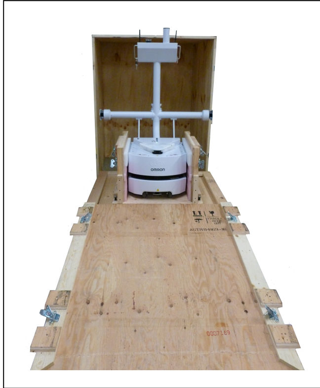
Figure 3-7. LD Platform Cart Transporter on Crate Base, with Ramp
