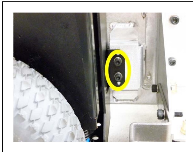
Figure 10-22. Mounting Screws at Bottom-Right of Drive Assembly
