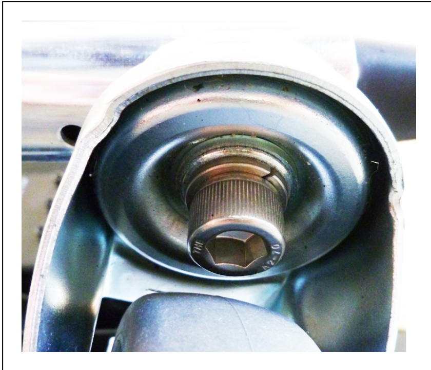
Figure 10-24. Front Cart Caster Screw Assembly
