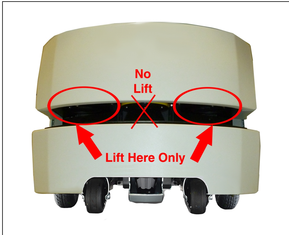
Figure 10-4. The Upper Surface of the Laser Slot. (A) Lift Here Only, and (B) No Lift
