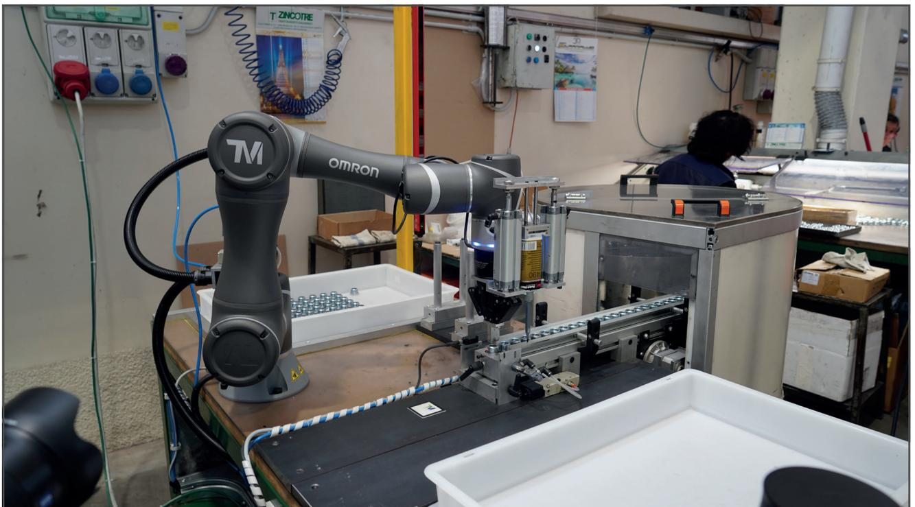
*The cobot takes care of the complete magnet assembly process - including applying the glue and inserting the magnets into the plugs.*
