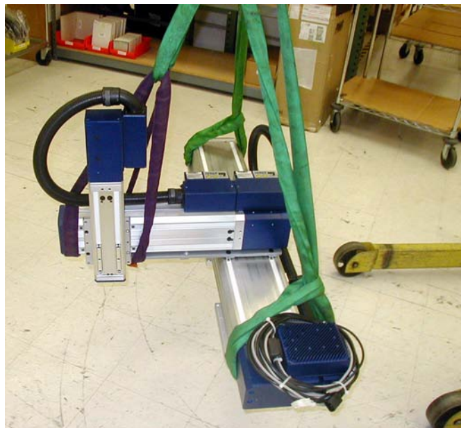
Figure 6-7. Lifting a Python System Using a Hoist and Slings
