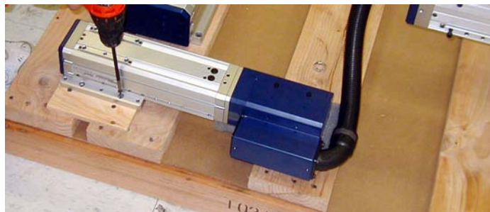
Figure 6-3. Removing Shipping Screws from Axis 3
