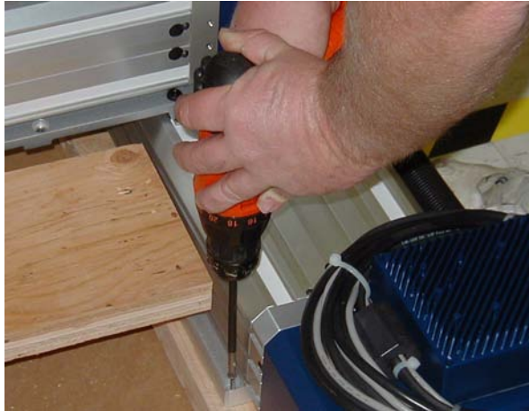
Figure 6-6. Removing Shipping Screws from Axis 1
