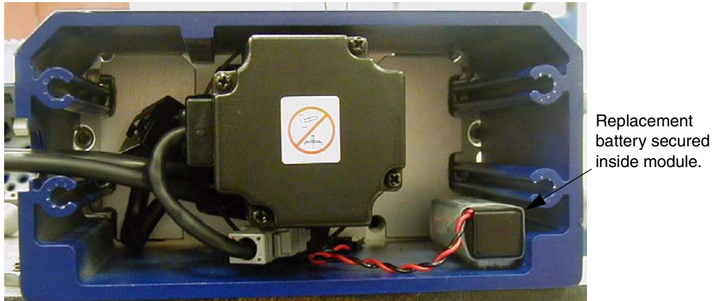
Figure 11-4. Replacement Cable Assembly Installed in Module
