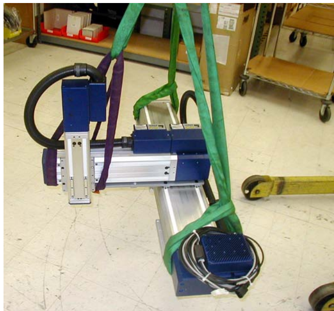
Figure 6-1. Recommended Lifting Technique for Python System
