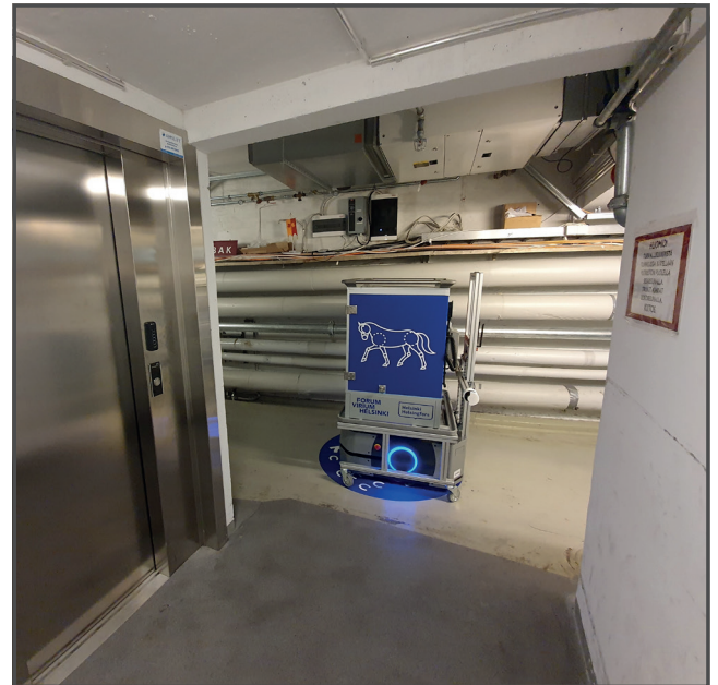
The mobile robot navigates independently along Kustaankartano's service tunnel, lifts and ramps.
