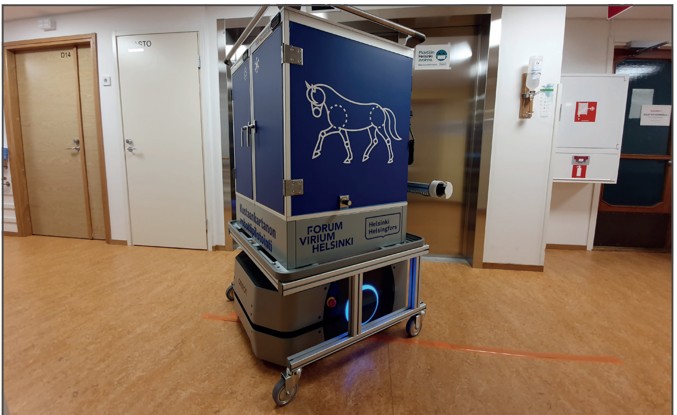
The mobile robot acts like a serving trolley, but as well as transporting meals and serving dishes, it can also be used for other items, such as mail.
