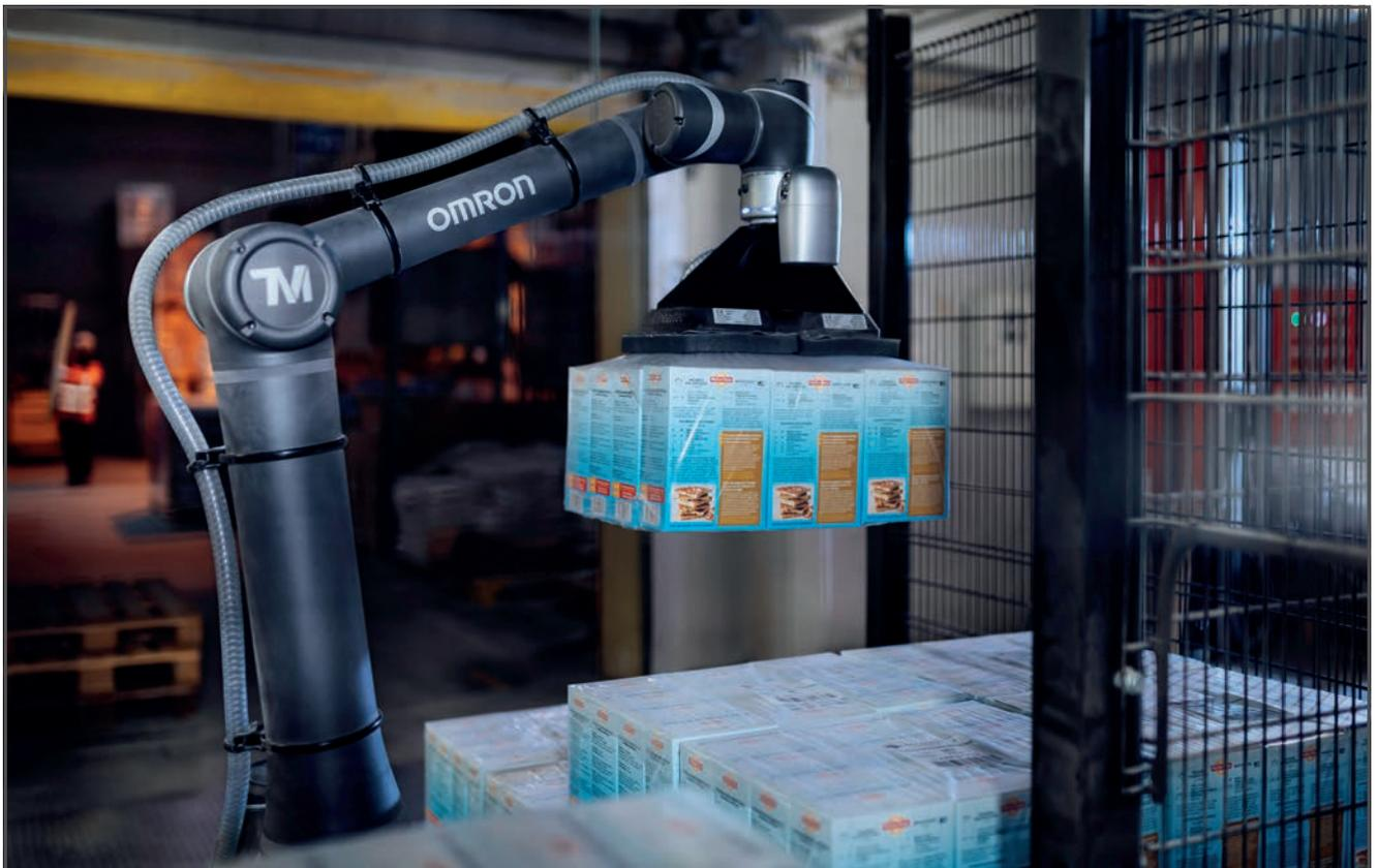
The OMRON TM12 has best-in-class reach and payload functionalities, as it can reach up to 1300mm with a payload of up to 12kg, and with a typical speed of 1.3m/s. It provides a flexible, high performance, automated solution for manufacturing operations. The cobot comes with integrated safety features and an inbuilt vision system. The integral camera can recognise objects under almost any lighting conditions.
