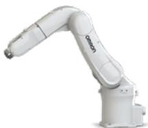
**Articulated Robots:** This type of industrial robot has multiple rotary joints, similar to a human arm. They offer a high degree of freedom and flexibility, making them suitable for inspecting assemblies with complex shapes or hard-to-reach areas. Articulated robots can be programmed to perform inspections from various angles and orientations.
