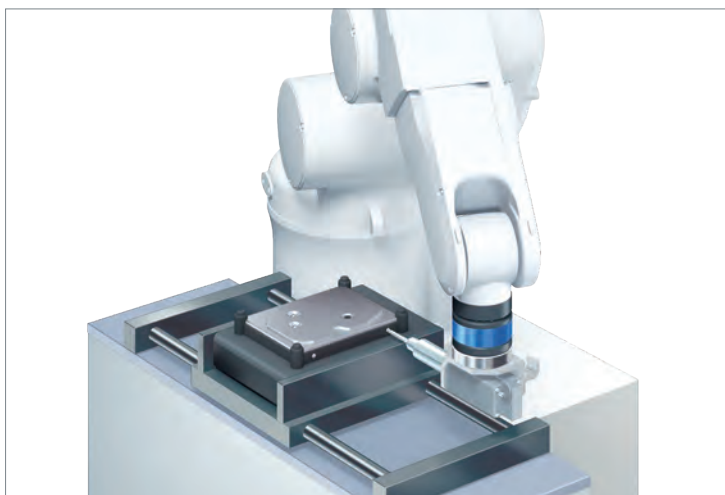
Screwing in horizontal direction
